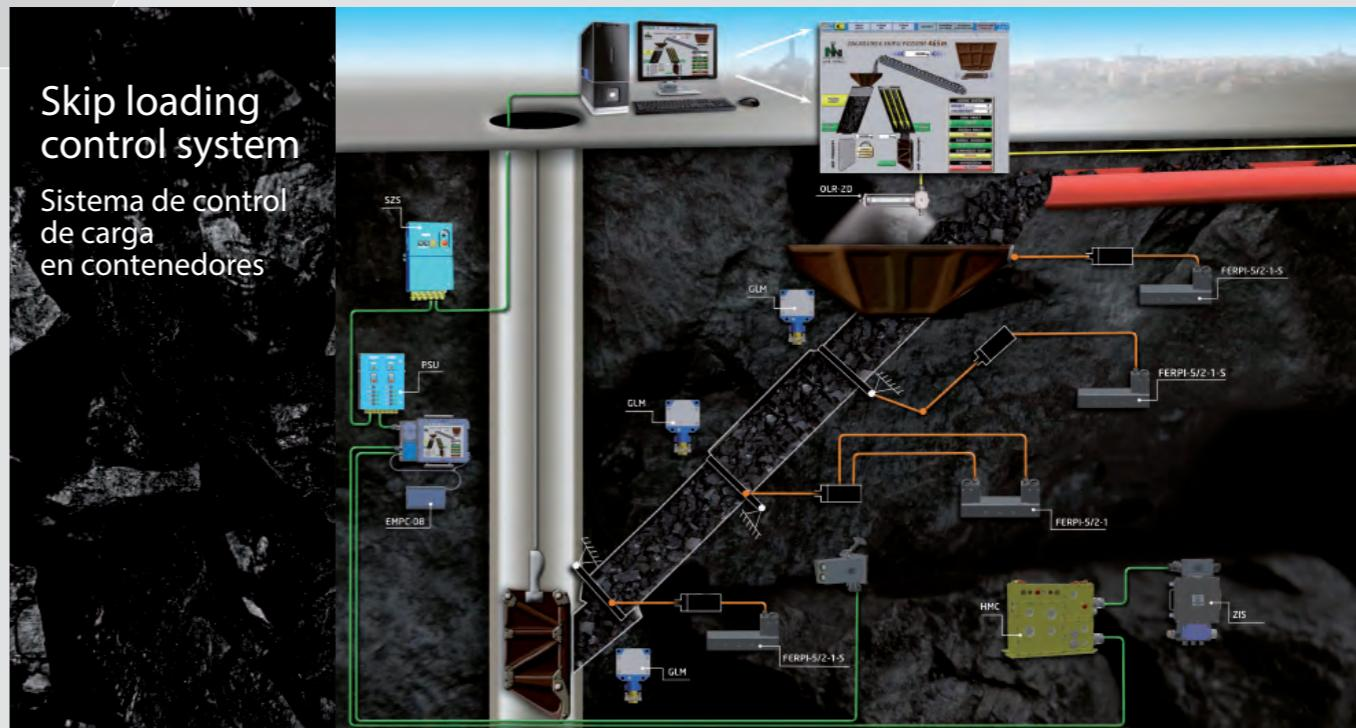
Skip loading control is one of the most important applications of our control suite. The system is based on a full controlled and monitored path from belt conveyors up to the skip loading for vertical extraction.
