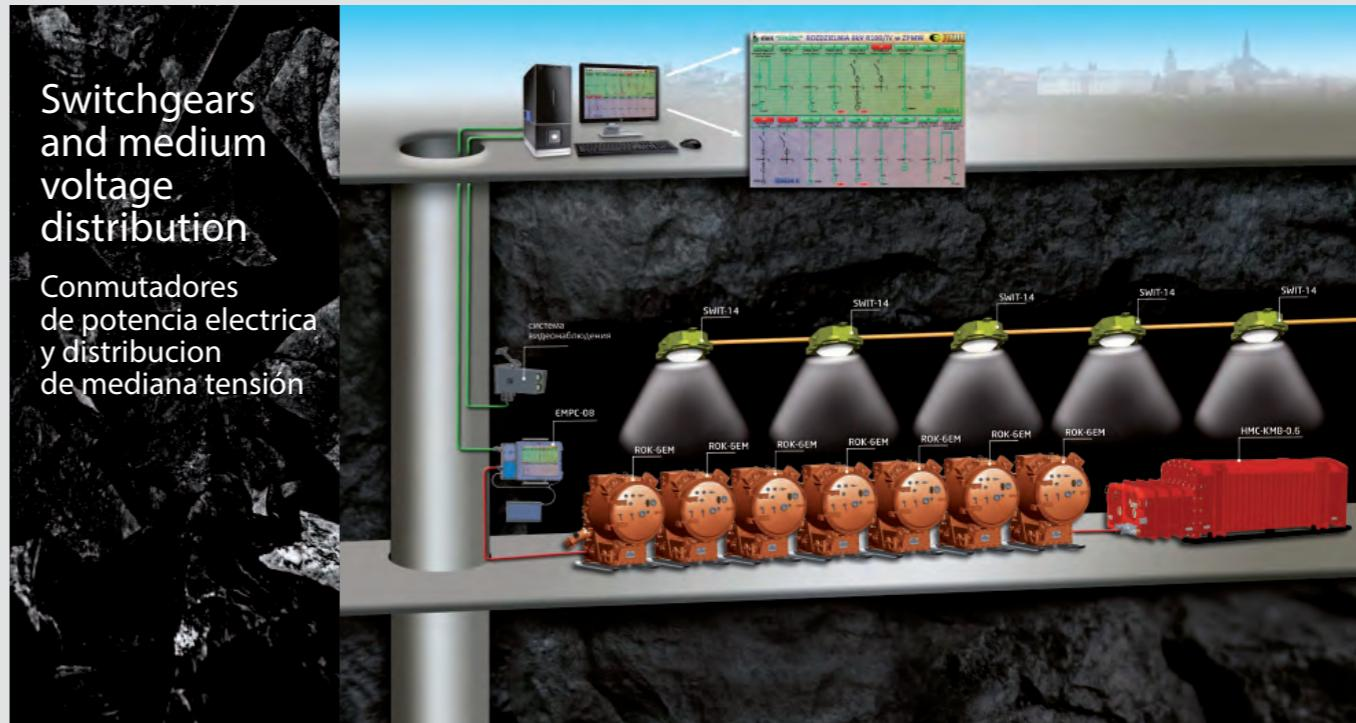
Our portfolio provides with a full range of medium voltage flameproof switchgears as well as transformers, equipments for improving the power factor, power supplies and drivers for controlling heavy machinery.
